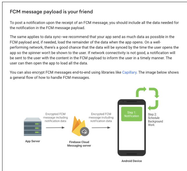
Figure 3: Google’s guidance to send as much data as possible via FCM payloads, noting that end-to-end encryption can optionally be used via additional libraries [69]. It is unclear whether the data flows labeled “encrypted” refer to this option or the fact that the transmissions use TLS.
